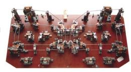
of some sections and ejection of parts on each jig station are provided. The jigs required close tolerance and location specifications and all location points in contact with the wires are insulated from the base. All electrode points are connected to a common copper base for weld electrical circuit completion.
