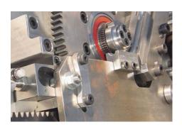
A pneumatically driven rack turns a pinion, with the tooling mounted directly on the pinion to maximise rigidity and strength. This unique design uses a second rack and pinion to ensure the pressure die 'rolls' around the periphery with no slippage; which together with highly polished contact surfaces, preserves the part surface finish.
